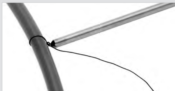
Fig. 4: The completed knot, pushed into place.
